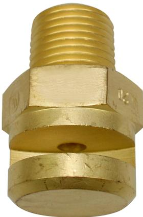
Reliable Models B Open Window, FM Open Window and FM Open Cornice Nozzles are especially designed for external use. They are installed in locations where a blanket of water is desired over a predetermined area. Open Nozzle systems can be operated manually or by quick opening valves that are pneumatically, hydraulically or electrically controlled.
